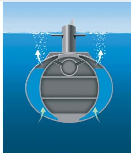
Figure 6 Controlling Density Using Ballast Tanks
