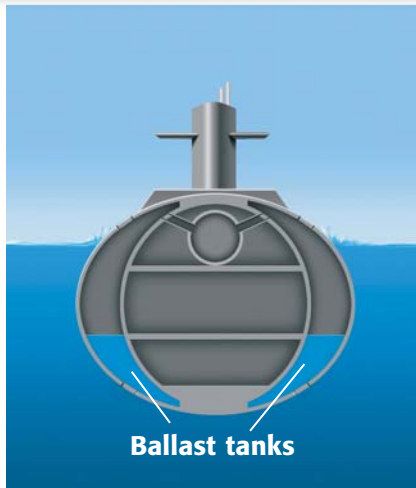
Figure 6 Controlling Density Using Ballast Tanks
