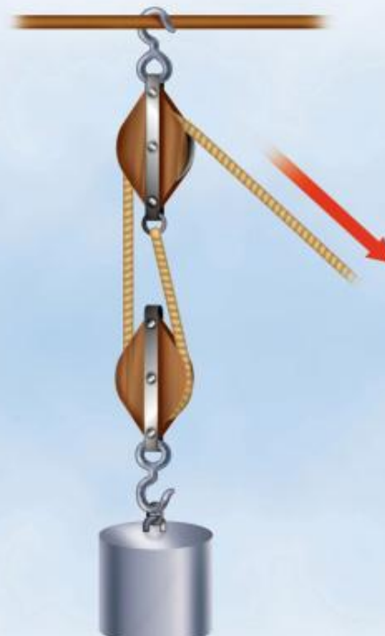
Pulley system I.M.A. = 2
