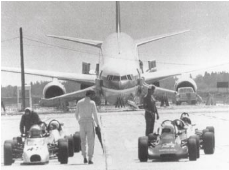
After both engines ran out of fuel, Flight 143 glided powerless for 29 minutes before the pilots brought it down on the end of runway 32. With a collapsed nose gear and two blown tires, the plane skidded to a stop just before hitting a telephone pole and a fence. The giant aircraft miraculously avoided skidding into people who were watching a sports car race on the abandoned runway.
